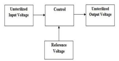
Fig 1 Block Diagram of Voltage Stabilizer
