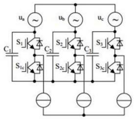
Fig.2 Three-phase differential AC chopper.
